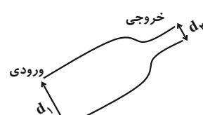
$$A_1 v_1 = A_2 v_2 \xrightarrow{\frac{A}{\pi d^2}} \frac{\pi d_1^2}{4} \times v_1 = \frac{\pi d_2^2}{4} \times v_2$$
